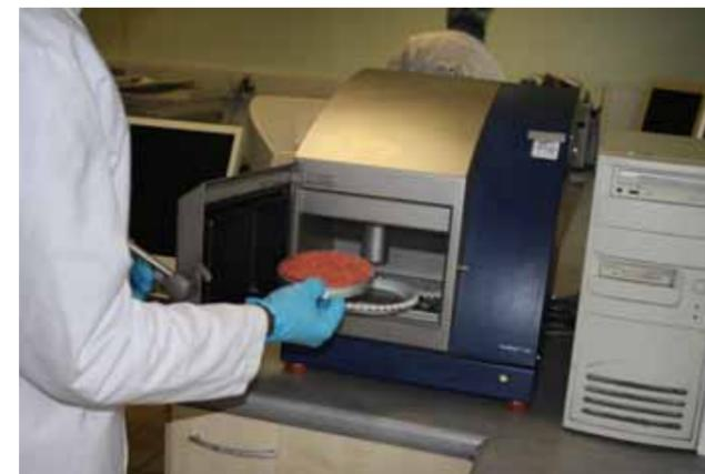
The FoodScan is used for a final, pre-release check testing for fat, salt, moisture and collagen in a single measurement taking less than a minute
